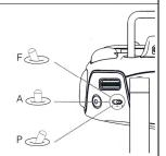
P mode (Positioning): P mode works best when GPS signal is strong. There are three different states of P mode, which will be automatically selected by the Inspire 1 depending on GPS signal strength and Vision Positioning sensors:
